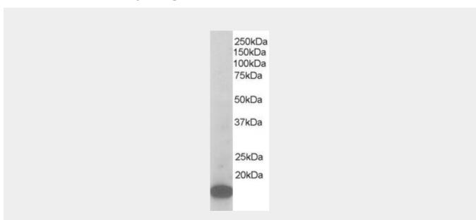
AF1110a staining (1  $\mu$ g/ml) of Mouse Brain lysate (RIPA buffer, 35  $\mu$ g total protein per lane). Primary incubated for 1 hour. Detected by western blot using chemiluminescence.
